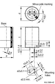
Snap-in terminals, length (6.3 + 1/-1.4) mm. Also available in a shorter version with a length of (4.5 - 1.4) mm. PET insulation cap is positioned under the insulation sleeve. Safety vent on the case wall.
